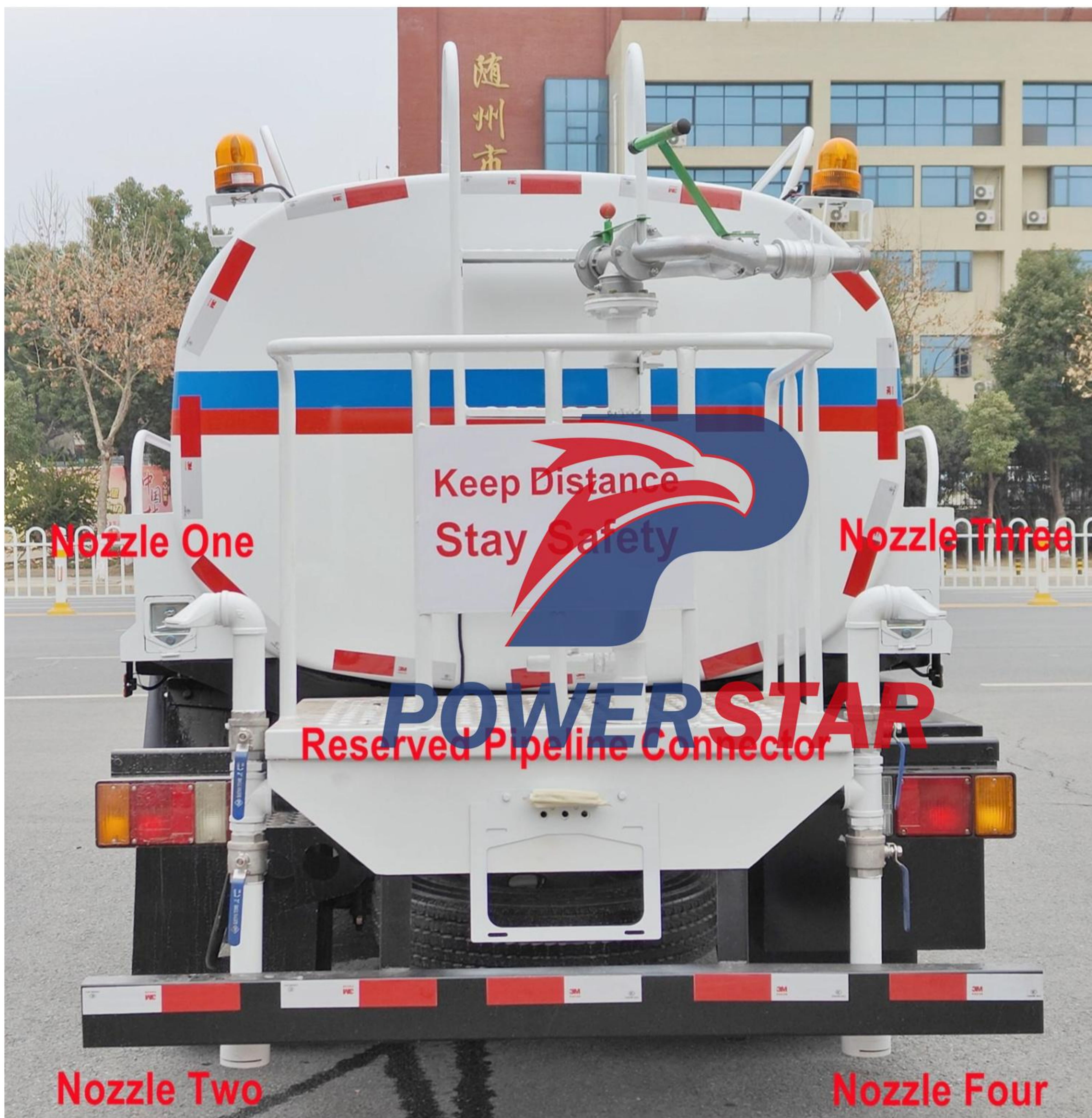
Rear Spraying Monitor: Rotation the front control valve to choose water spraying forms
